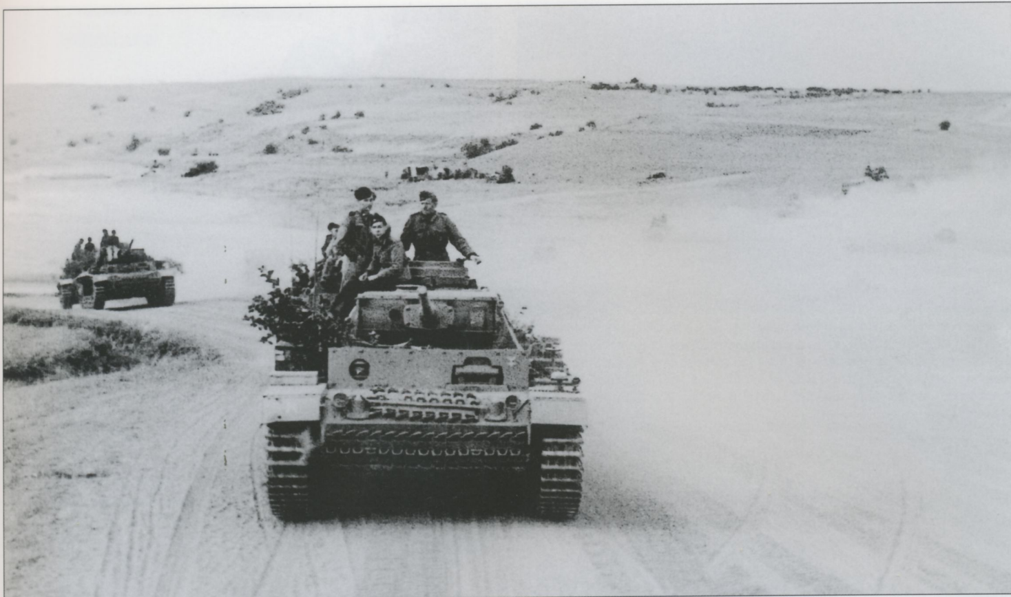
A column of Pz.Kpfw. IIIs from Panzergruppe Kleist advance towards the Volga during August, Drang nach Osten (Drive to the East). The lead tank is a 5cm gun-armed Pz.Kpfw. III Ausf. N with add-on 30mm armor bolted to the front of the driver's compartment. This additional armor was a lesson learned from North Africa. These tanks were also provided with thin spaced armor on the front, but the obvious bolts indicate the thicker add-on armor.
